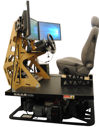
Figure 1: Cockpit mockup on the motion platform.
